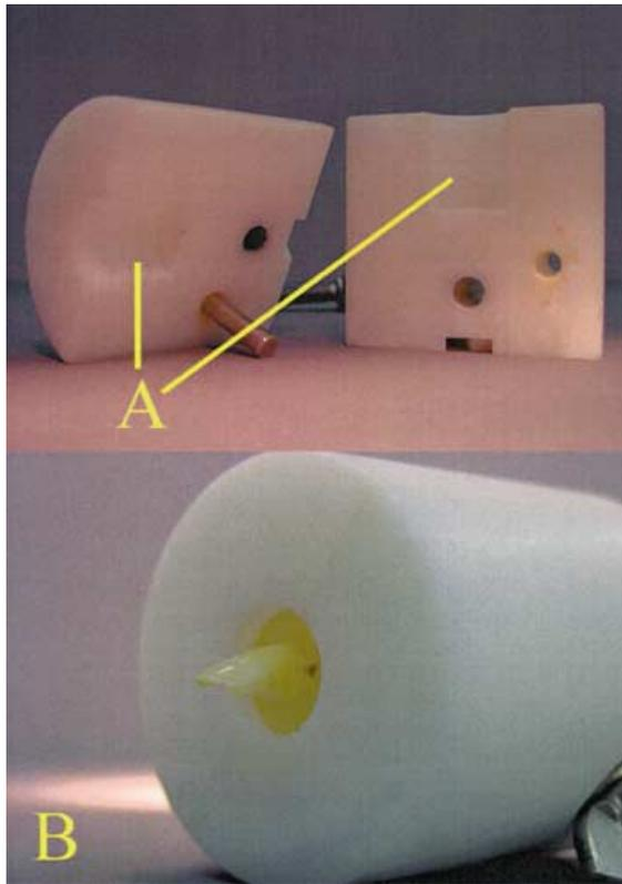
**Figure 1** Grooves in the walls of the muffle mould (A) allowed removal and exact repositioning of the complete tooth-block or sectioned parts of the tooth. A mandibular incisor was embedded in acrylic resin in the muffle mould (B).
