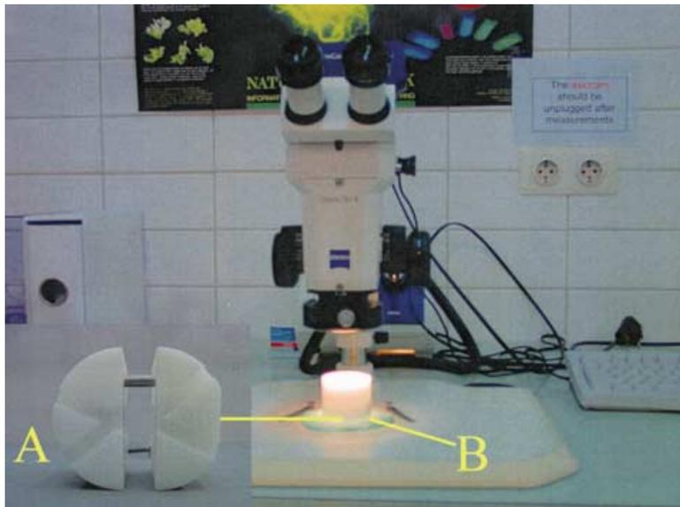
**Figure 2** The bottom of the mould was milled (A) and it was fixed to the microscope table with putty (B).
