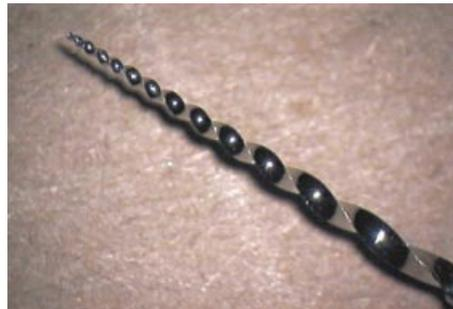
**Figure 15** 0.06 taper GT file with variable-pitch flute angles. Note the open, reamer-like flute angles at the shank end of the file, and the closed K-type flute angles near the file tip.
