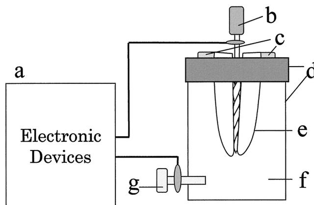
FIG 1. Experimental setup. (a) Electronic devices: impedance analyzer or Root ZX. (b) #1 Profile. (c) Self-curing resin. (d) Specimen bottle. (e) Tooth. (f) Saline. (g) Stainless-steel screw.
