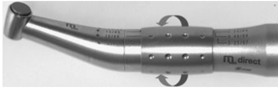
Figure 1 The swivel type adjustment ring of the Mtwo direct handpiece for selection of the different torque settings. Notice that the eight different settings which are located at the left and the right side of the adjustment ring are coded according to the taper and the size of the eight different Mtwo instruments. Thus, the settings for every Mtwo instrument are marked on this handpiece.
